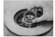
Step 3: A 3/8" spacer is installed at the lower front of the spindle between the steering arm and spindle to keep the steering arm parallel with the spindle.
